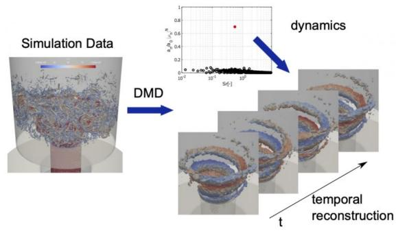
Figure 2: DMD analysis performed on the flow field of a turbulent flame. Instantaneous flow field (left), Spectrum of the DMD (top), Reconstruction of the dominant DMD-mode (right).
