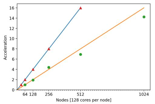
Strong scaling for turbulent channel (tri) and rocket engine simulations (circle). Performance (symbols) versus ideal (line) acceleration.
